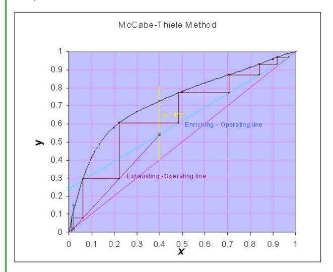
Number of theoretical plates are estimated from the McCabe-Thiele graphical construction method and found to be equal to 6.8
